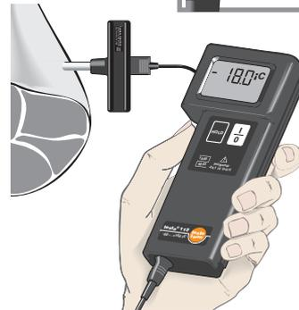
1 to 2 mins until the measured value has stabilised.
