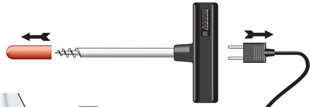
"Screw" the probe into the frozen food. The probe should reach the core of small pieces of frozen food and should be inserted at least 80 mm in large food. Never screw the probe in as far as the handle. 1
